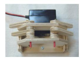
Using two of the 35mm long brass pivot wires assemble the links (Fingers) and spacers to the Palm at holes BB CC.
