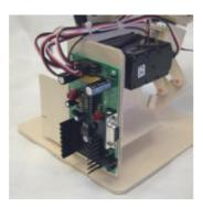
Fasten the controller board to the rear of the body back- piece 4 sheet 24- using 4 #2x3/8 screws. Connect the servo leads to the 3-way headers on the controller board- it doesn't matter which servo goes to which position- just ensure the colour on the leads match those on the controller board.
