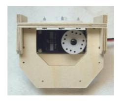
Fasten a large SO3 servo disc to the back of gripper part-3 using 4 #2x3/8 self tapping screws. Fasten an SO3 servo into the Palm using 4 M3x12 screws. Check the underside view and the servo orientation matches the above image.
