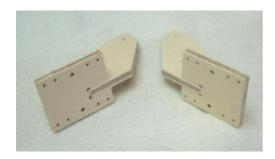
Glue together the 'Finger-tips' parts 10 & 11 (sheet 15) Note the two 'Fingers-tips' are handed and make sure that part-10 is at right angles to part-11.
