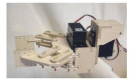
Connect a servo extension lead to the wrist SO3 and run it to its mid point using the controller. Position the Gripper assembly onto the servo so that the gripper is horizontal with the gripper servo uppermost. Fasten in place by threading the fixing screw carefully through the palm assembly.
