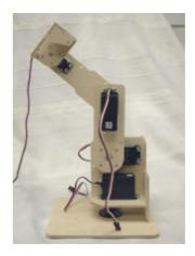
Fasten the SO6 servo to the other end of the forearm making sure that the servo shaft is towards the end of the limb, note that the SO6 servo is mounted differently from the other servos, see the drawing.
