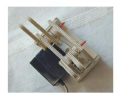
Connect the servo to a controller and check that the gripper opens and closes correctly, adjust the position of the disc on the shaft as necessary. Note that the effective length of the servo links is quite critical for the jaws to move symmetrically and the given lengths are measured to the centreline of the wire. If you have a problem make sure the finger cranks are on the correct pivots and that the servo links are the correct lengths and in the correct place, see the drawing.
