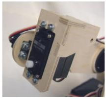
Insert an S03 servo into the wrist, with its output shaft towards the bottom and fasten in place.
