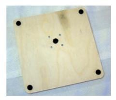
Fasten a large SO4 servo disc to one side of the Base plate (item 1 sheet 24) using 4 x #2x3/8 self tapping screws. Flip the Base and stick the 4 rubber feet in the corners of the base.
